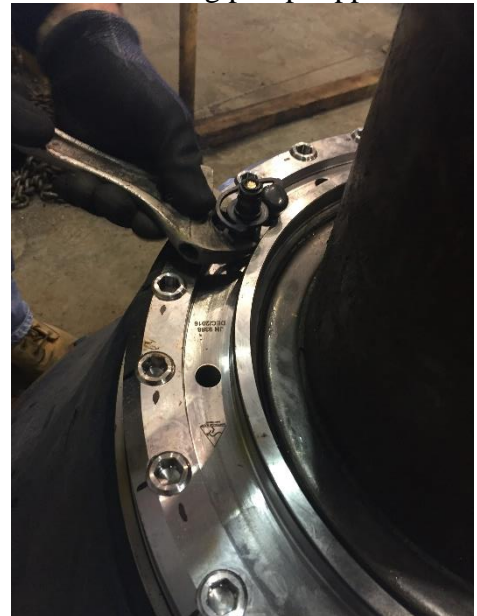
Releasing pump nipple
