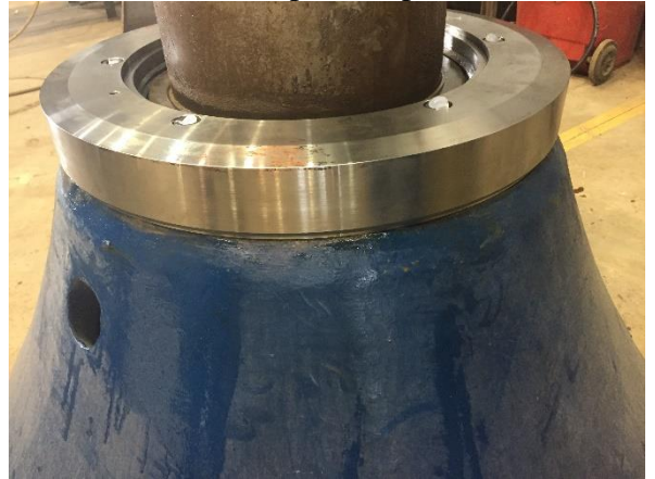
Sacrificial plate in position
