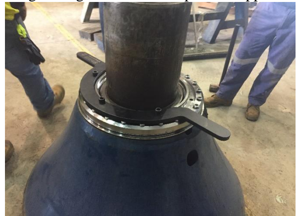
Tightening head nut with spanner supplied
