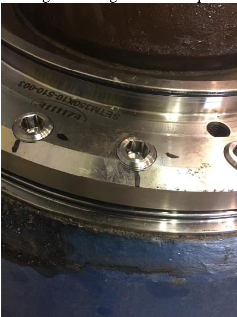
Jacking screws tightened in sequence
