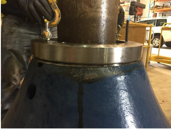
Sacrificial plate lowered onto head nut
