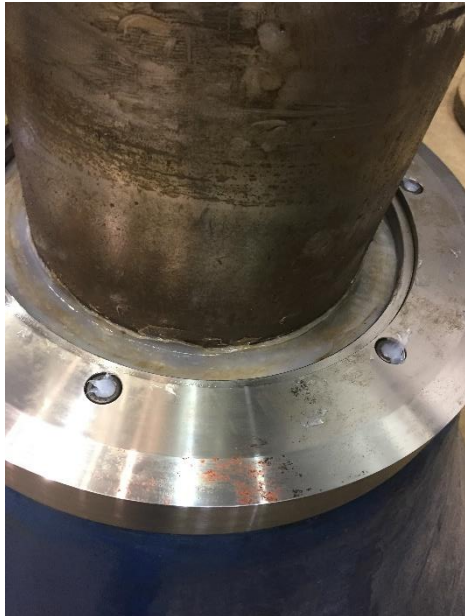
Bolt and inner race covered in silicone
