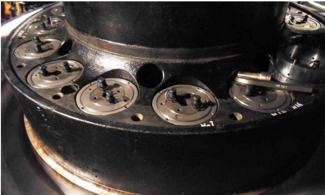
*Technofast EziTite M125 hydraulic bolts being used as an alternative to heater rods previously employed in turbine maintenance programs.*
