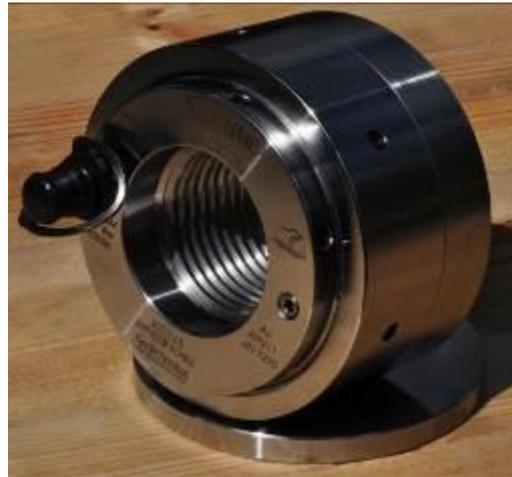
*EziTite® Hydraulic Nuts are rapidly applied by being placed onto bolt studs and hydraulically actuated to stretch the bolt to the precise tension required then locking it in place mechanically with a lockring. The reverse procedure permits equally rapid disassembly when it is eventually required.*
