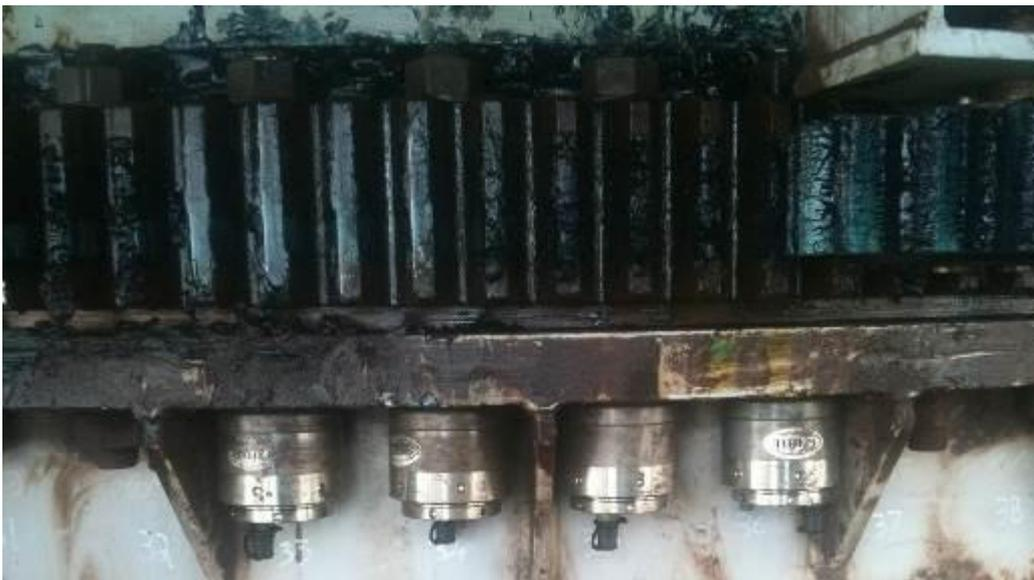
*Technofast EziTite hydraulic nuts, seen here fixed in groups of four, make assembly and disassembly tasks faster and safer and avoid downtime. .*
