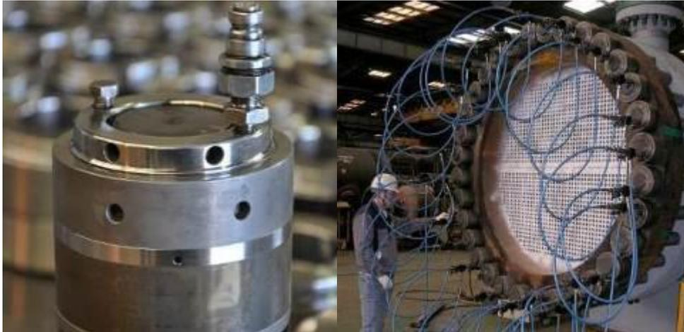
*Technofast EziTite TR high temperature hydraulic nuts, being installed on a Heat Exchange in refinery, makes assembly and disassembly tasks faster and safer and avoids downtime. .*
