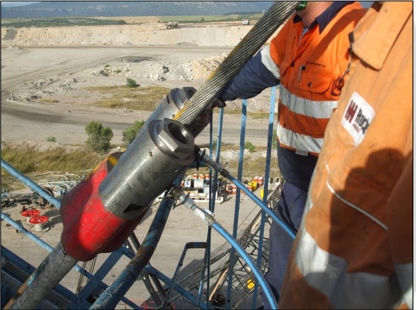
IBS Rope being tensioned with EziTite ® IBS EziTite hydraulic Nuts
