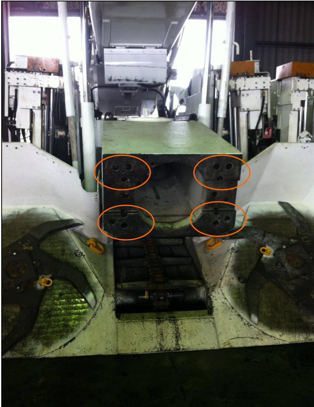
ABM25 continuous miner without boom installed showing bolt locations.
