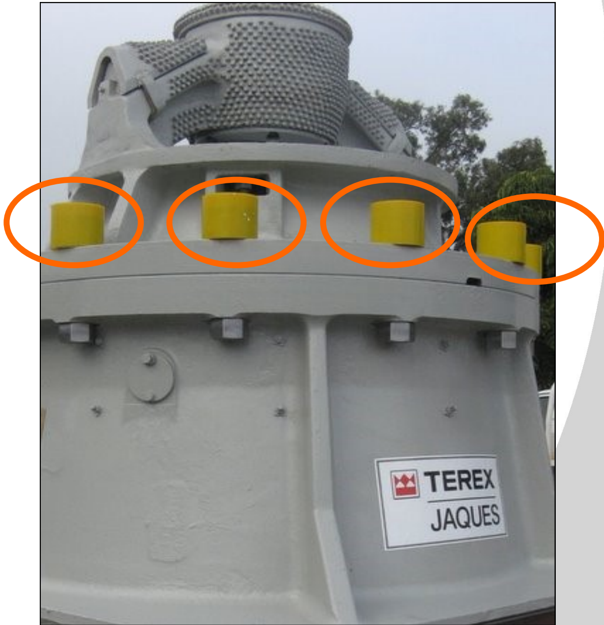
EziTite ® Hydraulic Nuts installed to and fitted with dust caps ready for service.
