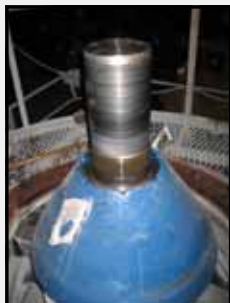
Mantle before the Installation
