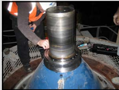
Mantle with Technofast's EziTite Hydraulic Head Nut installed
