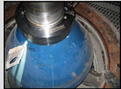
Close up of the EziTite Hydraulic Head Nut installed
