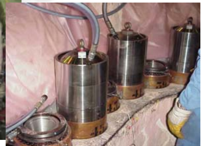
Special design Cone Nut & Matching Tensioner
